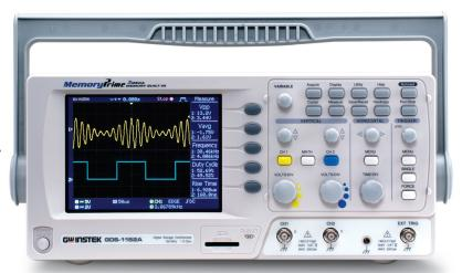
Additional automatic measurement functions incl. FFT and FFT rms
